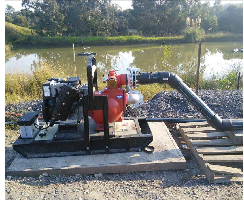
Veolia's timber recycling facility at Horsley Park is protected from spontaneous combustion by an Aussie self-priming four-inch diesel drive high pressure pump.
