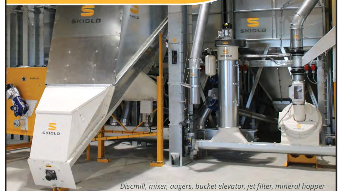
Discmill, mixer, augers, bucket elevator, jet filter, mineral hopper
