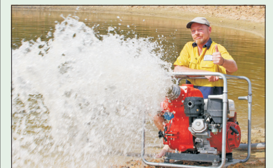
Aussie Pumps 4" trash pump moves dirty water fast.
